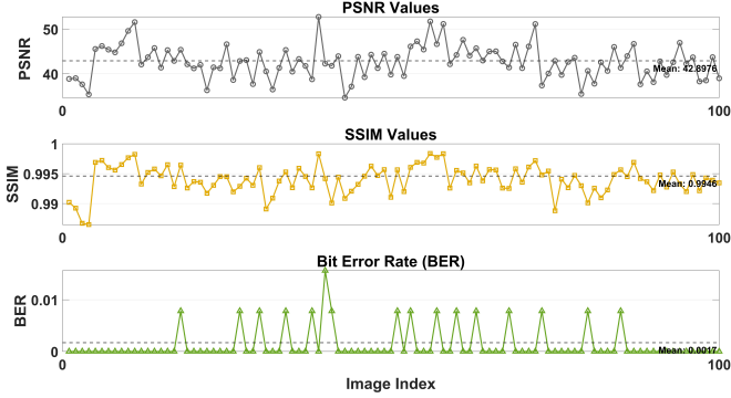
Fig. 7. Concealment assessment: PSNR, SSIM, and BER of the dataset.
